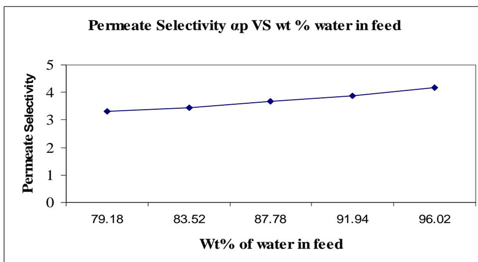
**Figure 3.5: Permeate Selectivity for Binary ethanol water mixture & effect of Wt% of water in feed**
