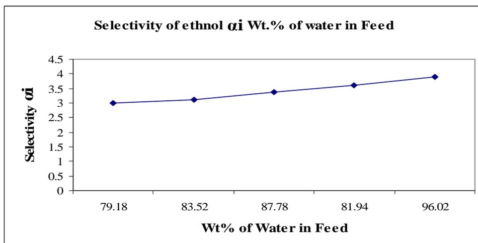
Figure 3.2: Ethanol selectivity for Binary ethanol water mixture & effect of wt% of Ethanol in feed
