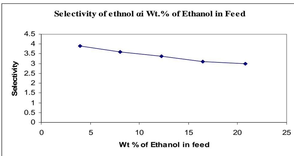
Figure 3.1: Ethanol selectivity for Binary ethanol- water mixture & effect of wt% of Water in feed
