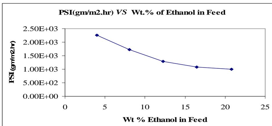
**Figure 3.6: Pervaporation Separation Index (PSI) for binary water-alcohol mixtures considering wt% ethanol in feed**
