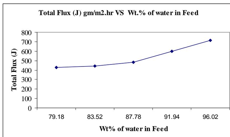
**Figure 3.31-Effect of Wt% of Ethanol in feed and Total Flux**
