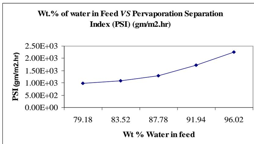
**Figure 3.4: Pervaporation Separation Index (PSI) for binary water-alcohol mixtures considering wt% water in feed**
