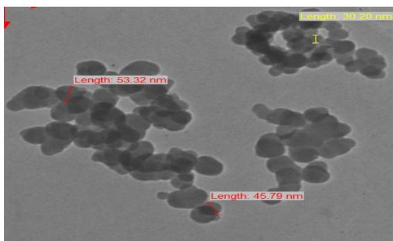
**Figure 3: Transmission electron microphotographs (TEM) of PANI-ZTP nanocomposite cation exchanger showing different particle size**
