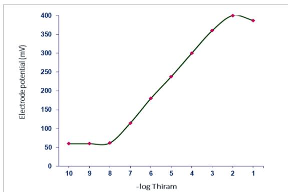
**Figure 6: Calibration curve for Thiram sensitive membrane electrode**
