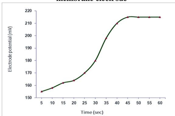
**Figure 7: Time response curve of Thiram sensitive membrane electrode**
