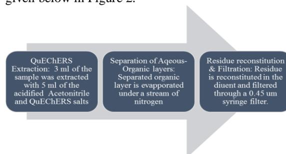
**Figure 2: Flow diagram of sample preparation**
