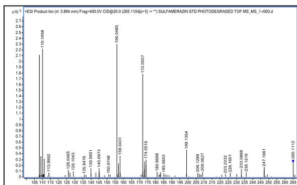
**Figure 10: Fragmentation pattern of Sulfamerazin eluting at 3.7 min**
