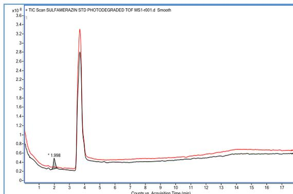
**Figure 7: Comparison of TIC of Control versus degraded sample. Degraded product at 1.998 min showing that it is more polar in nature (Color)**
