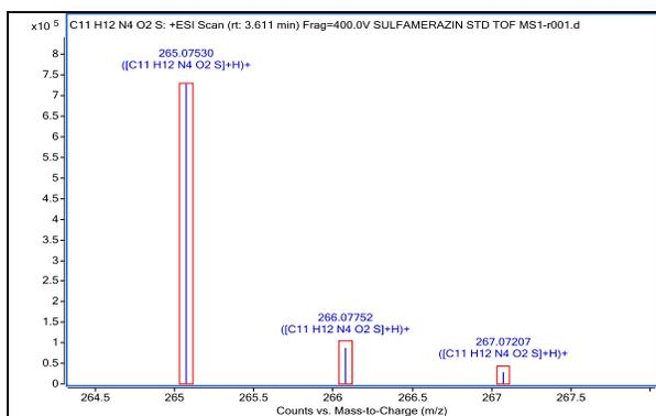
**Figure 6: Molecular formula generated from the measured m/z: 265.0753 and isotopic pattern by Molecular formula generator tool in MassHunter Qualitative software**
