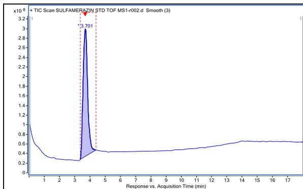
**Figure 5: Total ion Chromatogram of Sulfamerazin control sample**
