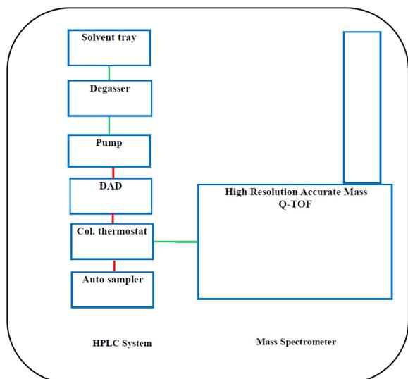
**Figure 3: Schematics of LC- MS/MS system used for analysis (Colour)**
