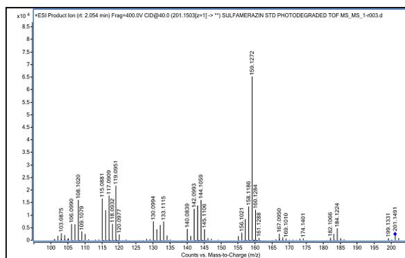
**Figure 11: Fragmentation pattern of Photo degraded compound formed and eluted at 1.99 min**
