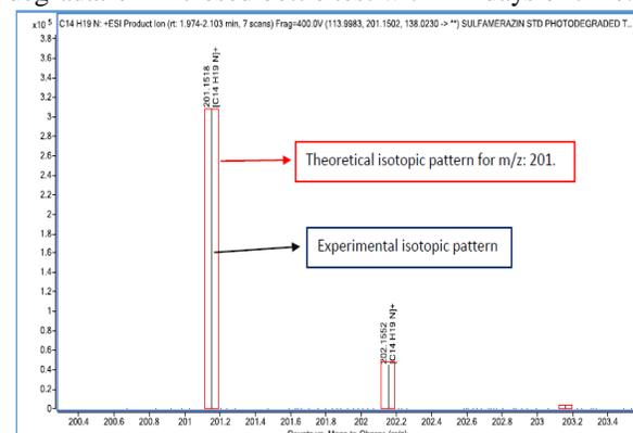
**Figure 9: Mass spectra of the degraded sample in TOF MS acquisition mode. The measured formula C<sub>14</sub>H<sub>19</sub>N can be seen in the figure (Color)**
