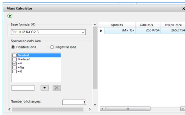
**Figure 4: Calculated  $m/z$  for Sulfamerazin in positive mode calculated by Agilent MassHunter Mass calculator**
