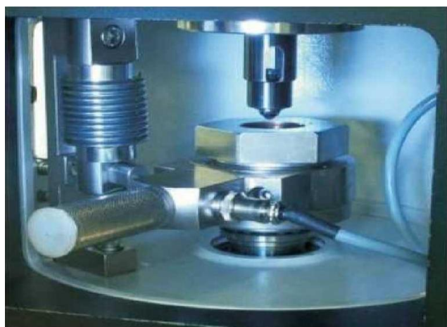
Figure 1: Ball pot assembly and Four ball testing assembly
